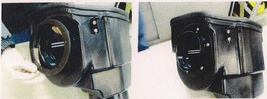
Step 8. Locate #3 "L" bracket. Install "L" bracket to Roto-Fab air box. Using the supplied 10-32 SS machine screws, fasten the bracket to the front side of the Roto-Fab air box. \*Note: Install the head of the machine screws from the outside of the air box.
