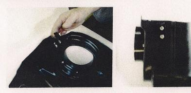
Step 9. Locate #14 Coolant Reservoir Bracket. Install the Coolant Reservoir Bracket. Using the supplied 10-32 SS machine screws, fasten the bracket to the back side of the Roto-Fab air box. \*Note: Install the head of the machine screws from the inside of the air box.
