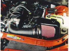
Step 13. Locate #2 Hood Seal. Install the air box hood seal. Using the supplied hood seal, install the seal around the top of the Roto-Fab air box assembly.
