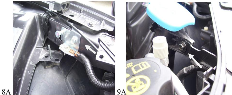
Step 9. Remove windshield fluid neck bolt. Using a 10mm wrench, remove the bolt shown in illustration 9A. The removal of this bolt is necessary for flexibility that simplifies the installation of your new air box.
