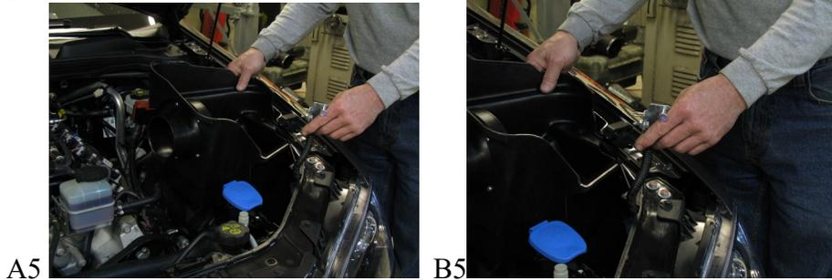
Step 7. Place the windshield washer fluid neck back to its original location and hand tighten the mounting bolt. Do not tighten this bolt at this time.
