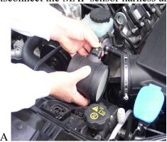
Step 6. Remove air box assembly. Using a 10mm socket, remove the two flanged nuts shown in illustration 6A. Pull firmly up on the airbox assembly and rotate as shown is illustrations 6B and 6C to remove air box.
