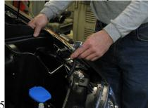
Step 7. Place the windshield washer fluid neck back to its original location and hand tighten the mounting bolt. Do not tighten this bolt at this time.
