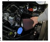
Step 13. Locate the #5 hose coupler, two of the #15 4" hose clamps, and the OEM MAF sensor. Install hose coupler onto the MAF sensor. Install and tighten hose clamp,
