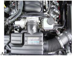
Step 5. Remove the MAF sensor. CAUTION be careful not to damage the MAF screen. Using a 7mm socket, loosen the remaining hose clamp on the MAF sensor. Pull the MAF sensor from the air box assembly. Using your fingers, squeeze and pull firmly to disconnect the MAF sensor harness and remove MAF sensor. Set aside for re-installation.
