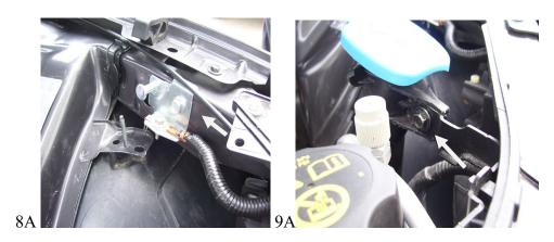
Step 9. Remove windshield fluid neck bolt. Using a 10mm wrench, remove the bolt shown in illustration 9A. The removal of this bolt is necessary for flexibility that simplifies the installation of your new air box.
