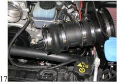
Step 17. Locate #8 4" Hump hose 3" long (this is the longer of the two 4" hump hoses) and two #15 4" hose clamps. Position clamps on each side of hump hose. Install hump hose assembly over the #17 hose sleeve on the MAF sensor assembly. Align the #8 hump hose with the edge of the #17 hose sleeve. See illustration on following page. Clock hose clamps equal to the previous installed clamps as shown in illustration A17 and tighten clamp to MAF sensor assembly.
