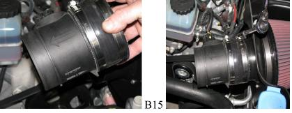
Step 16. Locate #17 3 3/4" x 3/4" hose sleeve. Install onto the MAF sensor flange. See illustration A16.
