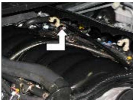
Remove the oil cap. Install the right side cover in the same manner as the other side. Make sure you are on the studs correctly before engaging the lower mounts.
