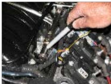
The engine cover mount for the driver's side rear mounts in the location shown. You should be able to push the wire loom downward out of the way of the engine cover bracket.
