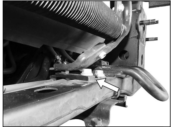
(Fig 14) Driver/left side of cooler relocated towards the radiator (arrow)
