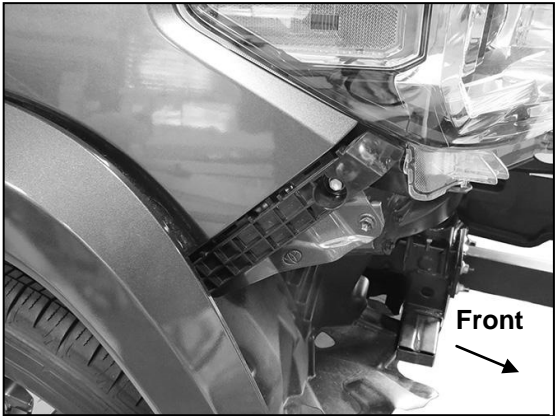
(Fig 5) Pull end of bumper cover outward to release from fender and below headlight. Remove hardware attaching top of bumper cover below grille and remove bumper cover
