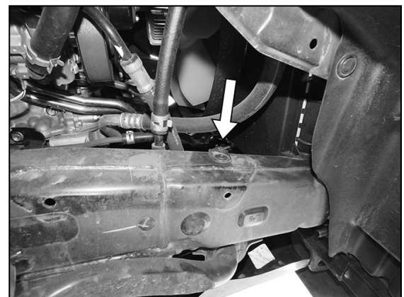
(Fig 11) Remove factory hex bolt attaching bracket to top of frame (arrow-bolt not pictured)
