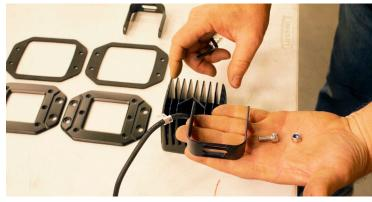
1. Using the bracket and provided hardware pictured above, attach the bracket to the light by placing the nut through the void in the heat sink fins. If needed, utilize a screwdriver to hold the nut in place while fastening.
