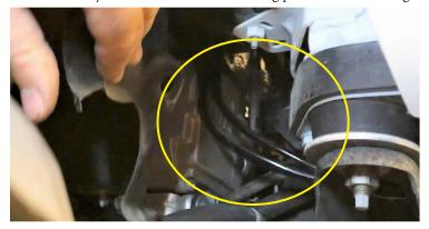
8. We chose to run the included kit wire harness through the bottom side of the engine compartment of our Jeep JL (closest to the battery) and out of the front end, between the bumper and grill. We gained access by peeling back the stock wheel-well liner.
