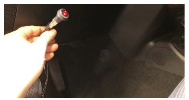
10. Run switch portion of wire harness through a safe area of the fire wall (available Daystar Fire Wall Boot part #KU20040BK). Do not run across any sharp edges or hot surfaces. Make sure that the wire is not in the way of the steering column, brakes, or gas pedals. Locate a convenient spot to place the light switch in the cab of your vehicle.
