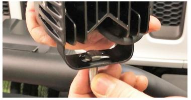
4. Hold the bolt down in the bracket anti-spin detents, during nut installation.
