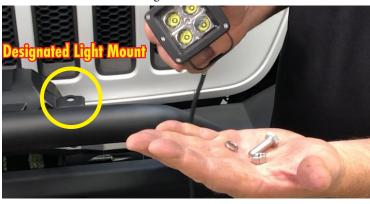
3. Utilize the provided hardware to fasten the light onto the two designated light points on the Scorpion bumper.
