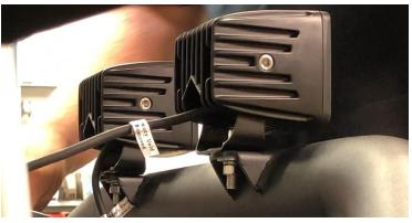
6. Fasten both lights to the Scorpion bumper using a wrench or socket.
