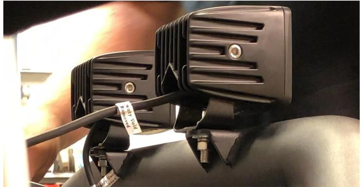
6. Fasten both lights to the Scorpion bumper using a wrench or socket.
