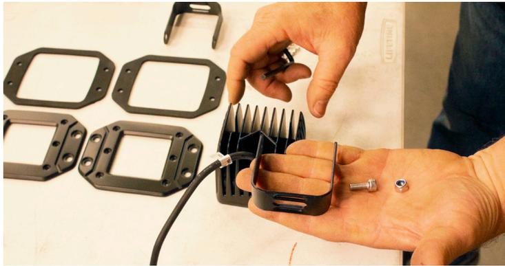
1. Using the bracket and provided hardware pictured above, attach the bracket to the light by placing the nut through the void in the heat sink fins. If needed, utilize a screwdriver to hold the nut in place while fastening.
