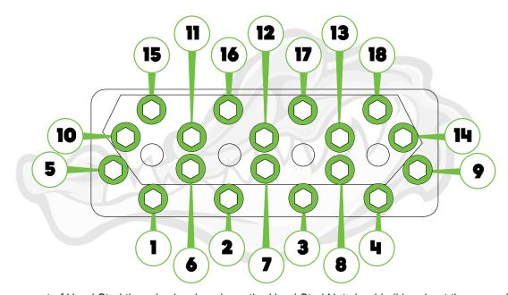
☐ The amount of Head Stud threads showing above the Head Stud Nut should all be about the same. If one appears to have more thread, the stud is most likely not all the way in the head.
