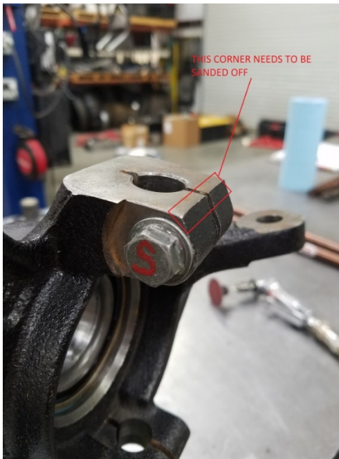
Figure 2: more detail shown of the area that needs to be removed, which must be done in both locations shown in Figure 1.
