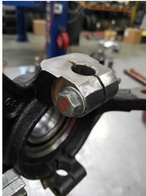
Figure 4: when done removing material this is what you will have, material removed right up to the flange of the bolt and nut.
