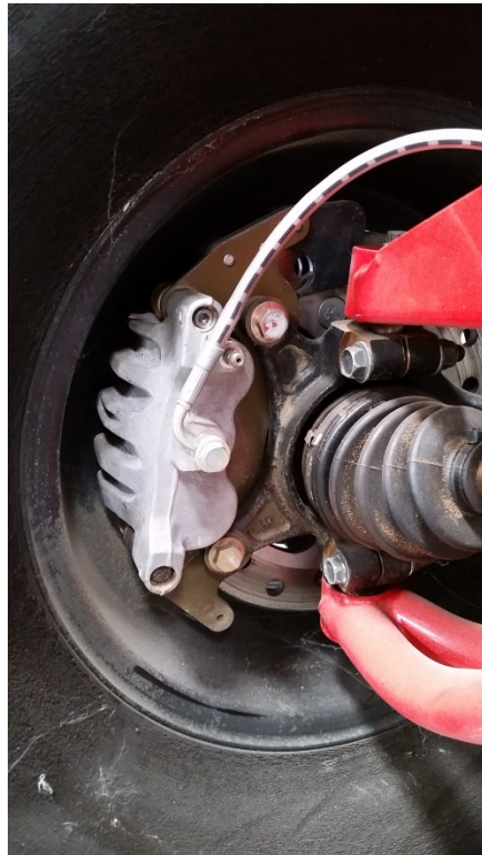
Figure 7: if there is a large gap like in Figure 6, crack the banjo bolt loose and turn and re-tighten like this Figure. Gives more room so the line does not rub wheel.
