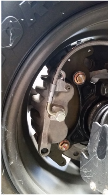
Figure 6: look at the distance from the line to the bleeder screw, this kicks the brake line up closer to the wheel, this is stock on some cars.
