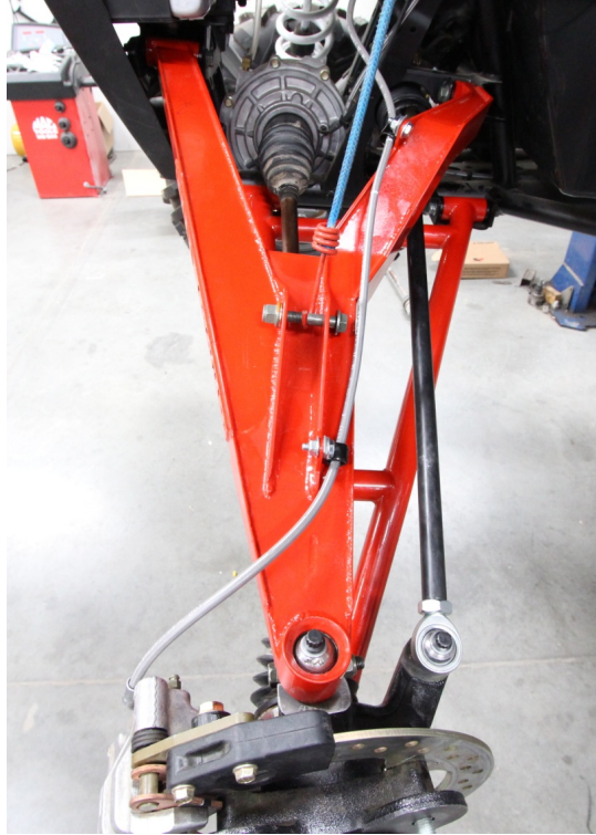
Figure 4: Fasten brake line with cushion clamps.
