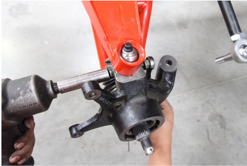
Figure 2: Tighten stud with pinch bolt.
