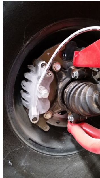
Figure 7: loosen the bolt a tad, just enough to turn the fitting closer to the bleeder as shown, retighten bolt.
