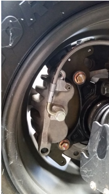
Figure 6: This is stock. The brake line fitting is far from the bleeder screw, this kicks the brake line up close to the wheel.
