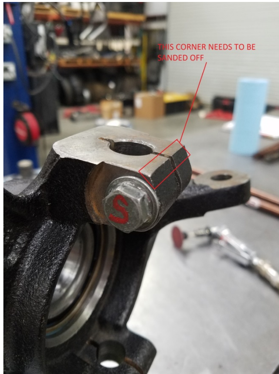
Figure 1.1: More detailed note of the trimming, which must be done to both areas shown in Figure 1.
