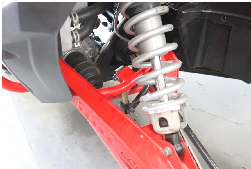
Figure 5: Stock sway bar bolts to the upper control arm just like stock.
