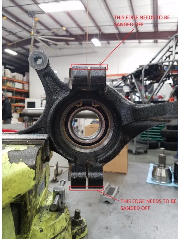
Figure 1: Notes show the 2 areas that will need trimming.
