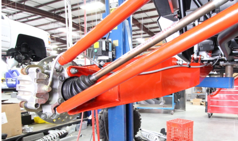
Figure 8: Installed brake caliper (notice brake line routing) and lower radius rod.
