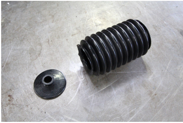
Figure 3: trim the small end of the dust boots off, so it can be attached to the clevis groove.
