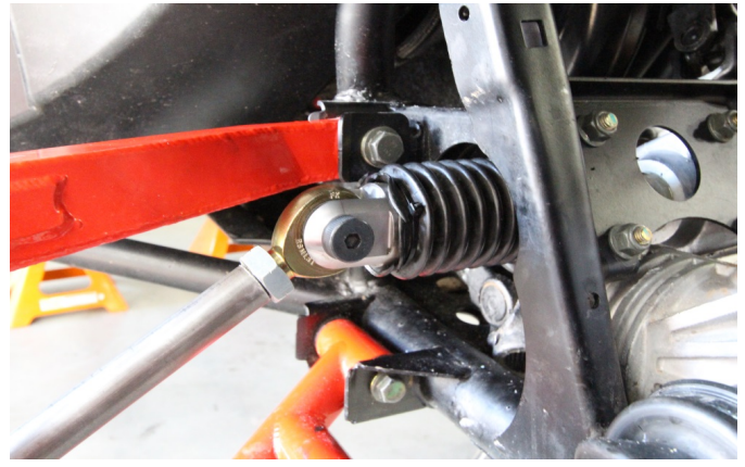
Figure 4: inner rod end attached to clevis, and dust boot tied to clevis groove.
