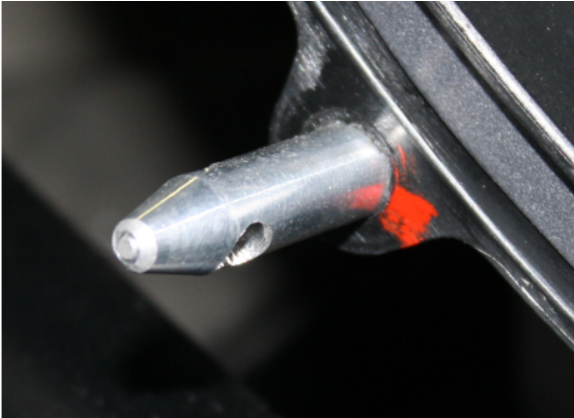
Figure 3: Pin Inserted into Hole After Drilling and Tapping
