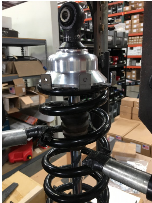
Figure 1: The shocks should look as pictured after installing the spring retainer and shock guard bracket.
