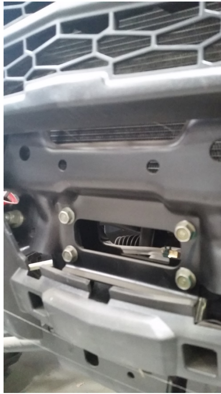
Figure 1: the stock frame holes that will be used, the bumper will be installed first and is not shown.
