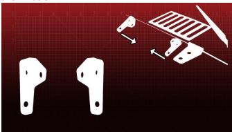
Begin screwing in the included studs into each bracket until it is flush on the underside. We recommend you use a threadlocker on each stud. Wait 10min for the gel to dry before installing your jack.
