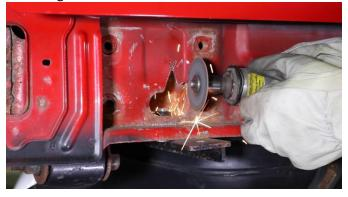
We found it useful to use a sawzall, die cutter, cutting wheel, and a dremel tool.
