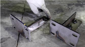
Hold the brace's rail up to the frame rail, inbetween the mounting bolt holes.
