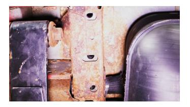
Secure the Brace using 3 of the included Hex Bolts, Lock Washers, and Flat Washers.
