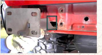
Trace the brace's rail dimensions onto the body, giving you a line to follow while cutting.
