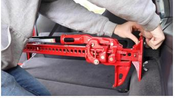
Repeat this with driver side and the 2" bolt and washers, while setting either the bolt to length by sliding it through the rail, or by adjusting the length of the jack.
