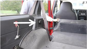
With an 8mm socket, remove the 3 bolts from each bracket, and set them aside to be used in the next step.
