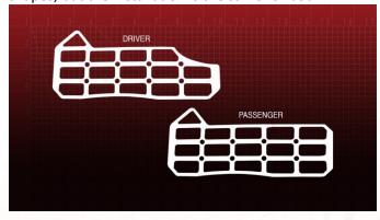
Hold the panel up to the base and align the edges of the two. With a marker, evenly mark 4 out of the 8 holes that are to be drilled.
