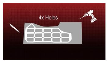
With a 5/16" drill bit, drill out the holes while being careful not to damage the inner lining.
