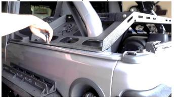
Depending on your preference or setup, the Tie Down will sit on top of any accessory, meaning the included knobs with secure it and anything extra.
