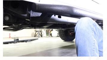
Insert the single M12 bolt and washer into the bottom of the rear most bracket with an 18mm socket. Tighten down each nut and bolt until the guard is tight against the frame.
