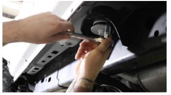
With an 18mm socket, remove the bolt from the driver and passenger side tube crossmember located just below each mirror.
