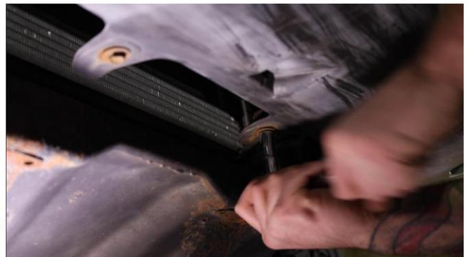
With a 10mm socket, remove the bolt below each headlight along the trim.
