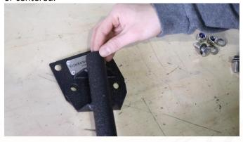
Assemble the mount with the 2 25mm hex bolts, 4 washers, and nyloc nuts with a 19mm socket and wrench.
