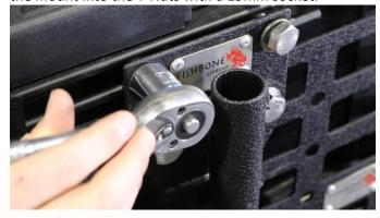
Install the flag into mount and secure it with the Wire Lock Pin.
