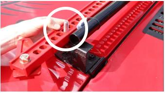
With the included bolts, washers, and wing nuts, secure the jack to the mounts through the rail.
