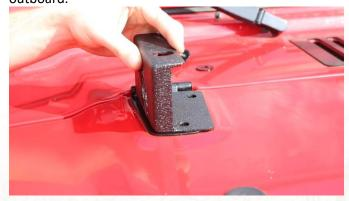
Remove the adhesive backing of one of the foam protectors and apply it to the bottom of the respective bracket. Place the bracket onto the hinge and secure using 3 of the included bolts and washer with a 5mm Allen key.
