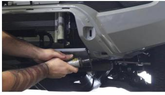
With the space now clear, with a 14mm socket, begin removing the 6 nuts securing the aluminum crossmember, and pull it away.
