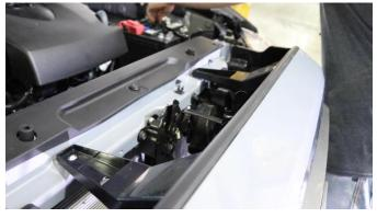
With a screw driver, remove the two push clips just inside the grille. Gently and evenly tug at the grille and remove it from the vehicle.
