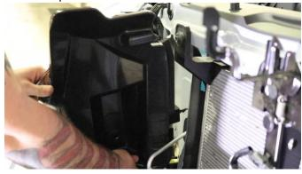
Gently pull at and remove the lower plastic bumper, followed by removing its support piece by pushing its retaining clips down.
