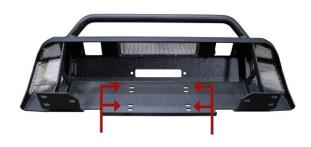
Lift the bumper into the opening and onto the factory frame studs, and secure it with the 6 factory nuts with a 14mm socket.
