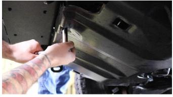
With the included bolt, washers, and nut, secure the driver side cooler bracket to the shown bracket hole, with an 11mm wrench.
