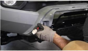
With your air saw, begin cutting around the crease and remove the trim.
