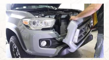
Remove the two remaining push clips from the air dams and pull them out.
