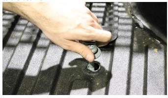
Next, with the remaining hardware, install the included stand-offs into the 5 upper holes of the panel so that the larger holes touch the plate, and the bracket pushes over the panel. Followed by installing the Bed Brackets into the bottom 8 holes so that the large spacing lines up with the bed bolt holes.
