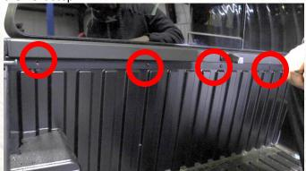
With a T-55 Torx Bit, remove the 2 bed bolts closest to the bed wall.
