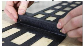
Next, secure the two panels with the 2 included bolts, washers, and nuts with a 10mm socket and 4mm allen key.
