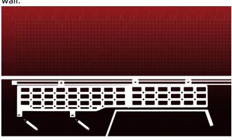
With a 23/64" drill bit, carefully drill these points. With a nutsert tool, install the included nutserts into these holes.
