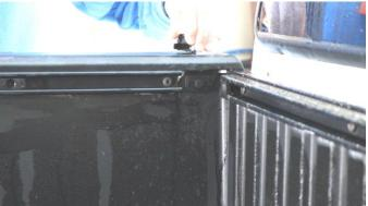
Remove the trail rail cap and insert the included T-Nut into it. Slide it to your desired location.
