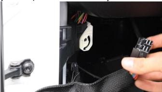
Next, remove the Torx bolt from the door hinges.
