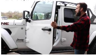
Begin by disconnecting each door's electrical connector, and unhooking the door strap. We recommend you roll your windows down before you do this, to make it easier to carry the doors.
