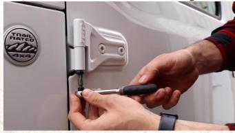
If you own a JL Wrangler or JT Gladiator, you will need at T-40 Torx bit for the inner door limiter bar. Each vehicle should come with their own door removal kit, which has these tools.
