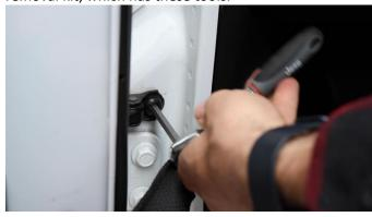
Lift your door straight up to remove the pins from the hinges. You may need to rock the door back and forth to get it to lift out. Store your doors in a safe place against a blanket or cardboard to protect the paint.
