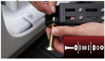
With a 17mm Socket and 17mm Wrench, tighten down the bolt and hex nut, while simultaneously setting the desired angle of the Foot Peg.
