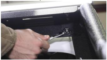
Begin securing the rack to the bed. Put 2 of the M12 carriage bolts through the bracket as shown, and rotate it into the side panel bracket, and up into the bed rail. With 2 flat washers, lock washers, and hex nuts, tighten the two brackets down onto the plastic rail with a 19mm socket.
