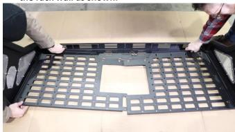
Follow the perimeter and loosely secure every bolt point with M6 bolts, washers, and flange nuts. Including the middle joined plates.
