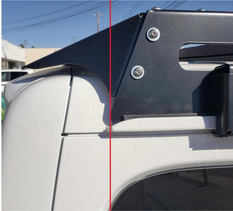
8. Install edge trimming on the edge of the 4 outer rail mounting plate lips.
