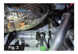
Remove the transmission fluid fitting bracket bolt on the side of the transmission case.
