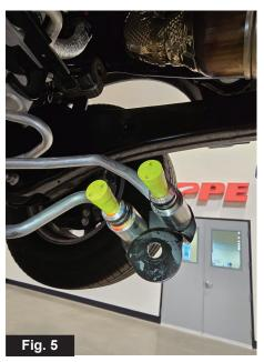
Remove the stock fill plug underneath the pan to partially drain the transmission fluid.
