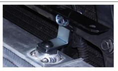
(A) Install cooler bracket bolts. Be sure to place the bracket with the oval hole at the top and the round one at the bottom.
