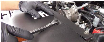
Remove retaining clips and radiator cover.
