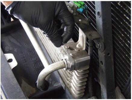
Remove the retaining clips and oil lines. Place towels or collection container below fitting to catch fluid.
