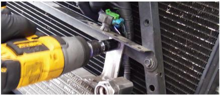
Remove bracket bolts and stock cooler.
