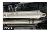
Step 6. Install the 4" Angled Pipe (C) with the 4" Exhaust Clamps (G). Secure hanger on the exhaust insulators. See (FIG 6 & FIG 7).
