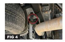
Step 4. Install the 4" Inlet Pipe (A) onto the factory exhaust system with the 3" Exhaust Clamp (H). Secure hanger on the exhaust insulators. See (FIG 5).
