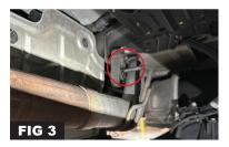
Step 3. Remove the stock exhaust from the exhaust insulators. See (FIG 3 & 4).
