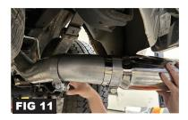
Step 10. Adjust fit and tighten all Exhaust Kit Clamps (G & H) starting from front to back.
