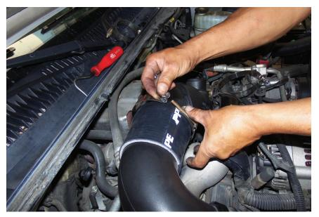
**STEP 16**Place clamps onto the cut silicone hose and tighten to fit.
