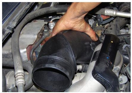
**STEP 7**Place intake duct into position.
