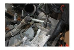
Disconnect EGR air intake (6 bolts and nuts). Move up and out of the way to make room for install.
