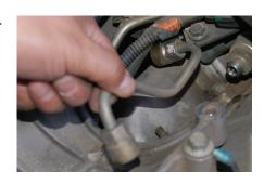
8. Remove factory fuel rail fitting using a 7/8 socket.
