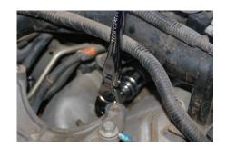
Lubricate the Ported Fuel Rail fitting with petroleum jelly, install and torque to 52 ft. lbs.
