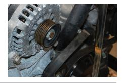
6. Disconnect power cable and plug from alternator.
