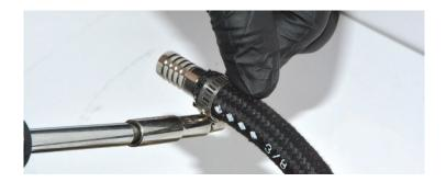
6) Connect adapter to fuel filter housing feed line. Tighten clamp.
