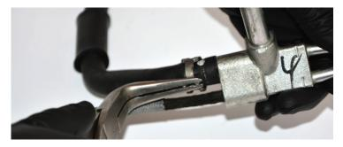
5) Install adapter on feed line hose and tighten clamp.
