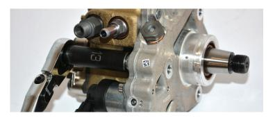
2) Reuse stock washer. Replace stock fitting with upgraded PPE Fuel Feed fitting. Tighten to 18 ft lbs.
