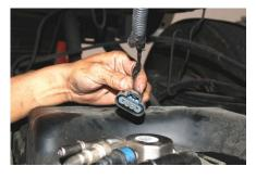
**Step 7**Disconnect sending unit sensor plug.
