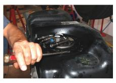
**Step 9**Remove sending unit from fuel tank (Be sure to drain fuel).
