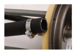
**Step 17**Lubricate 5/8in fuel line and connect to fuel pickup.
