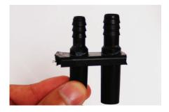
**Step 15**Drill .09375 (3/32in.)screw holes through plastic using fuel pick up as a guide.
