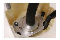
**Step 20**Secure 5/8in. hose using hose clamp provided in kit.
