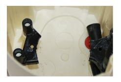
**Step 18**Install fuel pickup using screws and lock washers(Do not over tighten screws)
