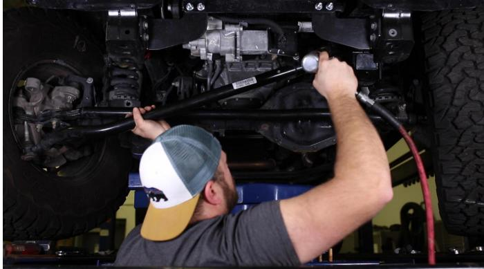
a. We recommended the use of an air hammer with pickle fork attachment for fastest and easiest removal. The joint will be taper locked into the pitman arm and will require a good deal of effort to remove.
