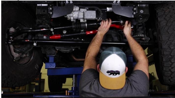
*i.* Note – clamps still only snugged - you will need to adjust this once everything is back together and the vehicle is on the ground (See Images for correct washer orientation)
