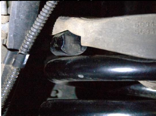
Figure 8: Top Spring Pigtail Installation
