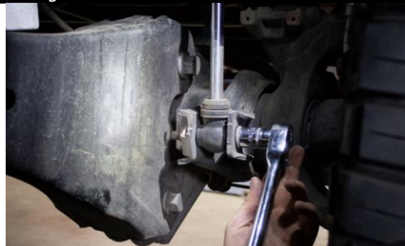
Figure 2: Front Shock Lower Bolt Removal
