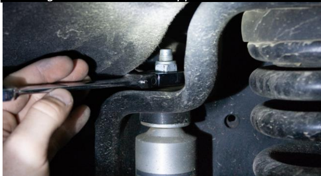
Figure 1: Front Shock Upper Nut Removal
