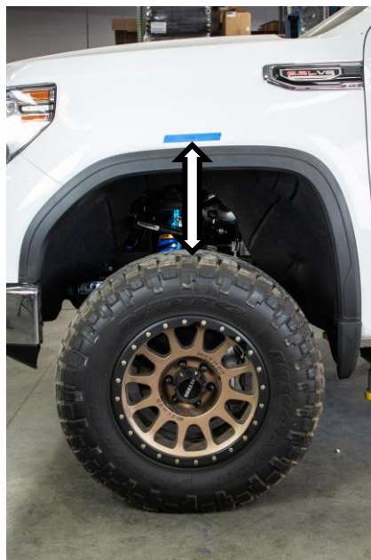
Figure 4: Measuring and Setting Ride Height
