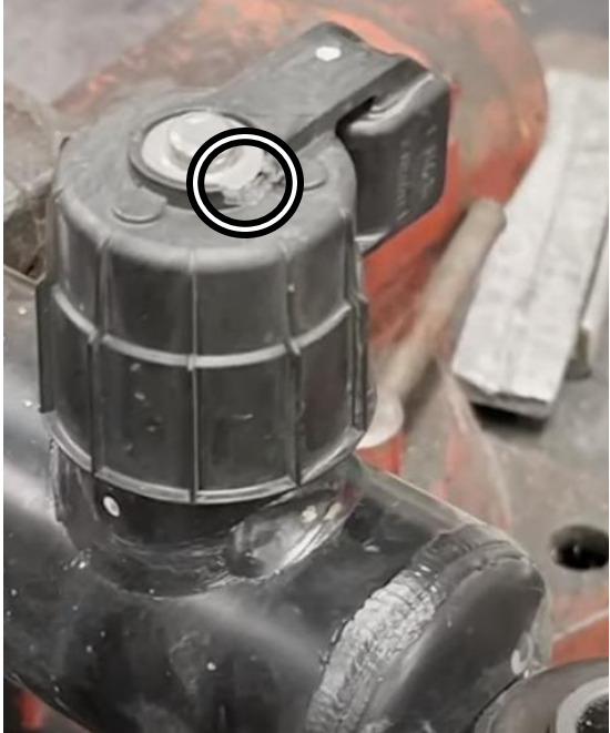
Figure 1: Cut or knock out the melted plastic retaining the cap.
