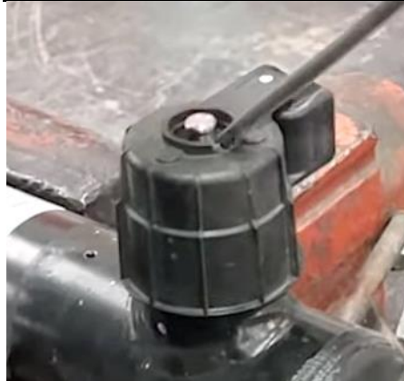
Figure 2: Remove small metal cap.
