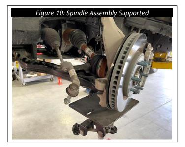
**12.** Remove the nut holding the UCA to the spindle and remove the UCA from the spindle. Ensure that the spindle does not fall over or put tension on the ABS sensor wire and the brake lines
