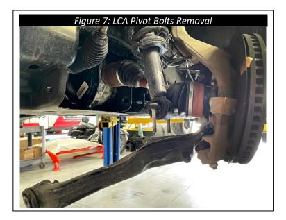
**9.** Remove the strut from the vehicle. Remove the 3x nuts on top of the strut to free the strut from the frame.
