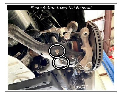
**8.** Remove the LCA pivot bolts. Swing the LCA downward and free of the strut. Place the hardware safely aside, it will be reused later.
