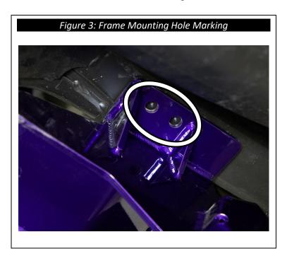
7. Either loosen the forward leaf spring mounting bolt and swing the frame mount bracket away from the frame or use the frame mount bracket as a drill template, and drill through the bottom side of the frame using a 1/2" drill bit, see Figure 4.
