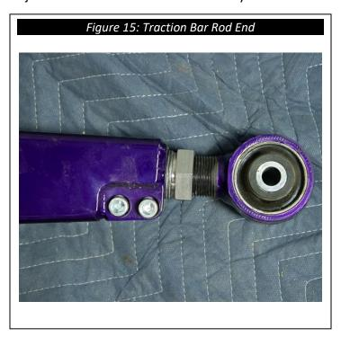
**20.** Locate <u>HP9205</u> and find one (1) 9/16"-12 x 5" bolt, two (2) 9/16" flat washers, and two (2) 9/16"-12 lock nuts. Install the traction bar end with the bushings between the frame mount bracket shackles, see Figure 15.
