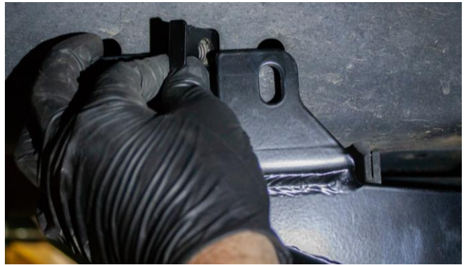
Figure 5: Insert Nut Tab
