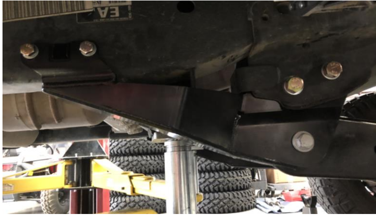
Figure 7A: Radius Arm Pivot Installed
