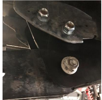
Figure 7B: Radius Arm and Drop Bracket Installed
