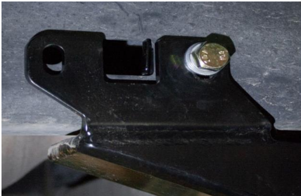
Figure 6A: Rear Mount Front Bolt Installed
