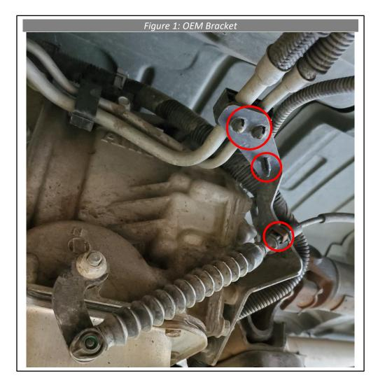
2. With all the wires, hoses, and shift cable loose from the cable bracket, remove the two bracket mounting bolts and OEM bracket. See figure 2. One of the mounting bolts is not visible in the image.
