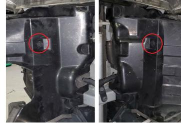
7. Using a trim removal tool, remove the two plastic push-rivets from the air dams.
