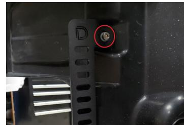
10. Loosely secure the brackets to the air dams with the provided M6 screw, washer, and nut.
