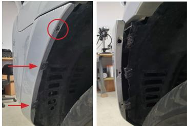
5. Using a trim removal tool, pull the upper edge of the bumper off the snap feature, and slide the lower two screw-clips off the bumper. Then pull the corner of the bumper away from the fender.
