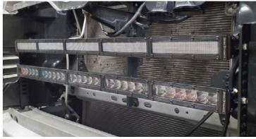
11. Install your Stage Series 30" light bars in the brackets with the provided flanged-head M6 hardware. For two bars, we suggest installing in the 1<sup>st</sup> and 6<sup>th</sup>, or 1<sup>st</sup> and 7<sup>th</sup>, slots from the top.
