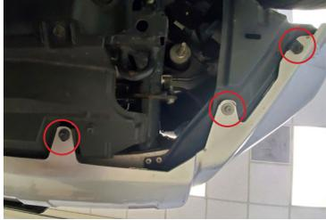
3. Using a 10mm socket, remove the six screws along the bottom of the bumper (passenger's side shown in picture to the left).
