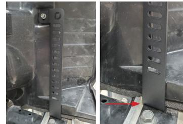
9. Slide the open-slot of your new Diode Dynamics Toyota 4Runner SS30 brackets under the air dams to the bolts loosened in the previous step.
