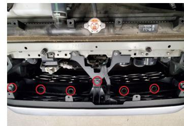
2. Using a trim removal tool or flathead screwdriver, remove the six plastic push-rivets shown in the image to the left.
