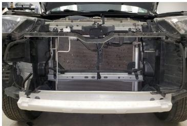
6. With help from a second person, pull the bumper straight forward to release snaps around the headlights and remove the bumper.
