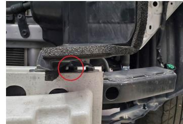
8. Using a 14mm wrench, loosen the second from the outboard bolt on the bumper bar (driver's side shown in picture to the left).
