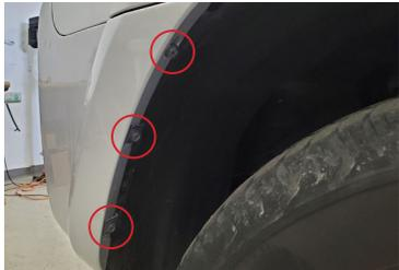
4. Using a 10mm socket, remove the three screws from the edge of the front bumper in the wheel well.
