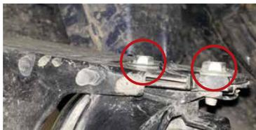
4. Pull the fender liner back and remove the two 10mm bolts holding the factory fog lamp in place. Remove the factory lamp.
