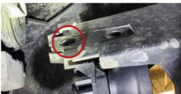
5. Install the SS3 pod and bezel onto the vehicle using the included 8mm hex bolt.
