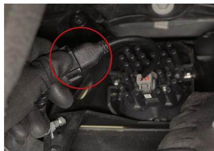
5. Plug the SS3 into the factory fog light harness using the included DT wire adapter. Test function. If the light does not turn on, try flipping the connector 180°. Install the retaining clip from the factory harness into the back of your new bracket.
