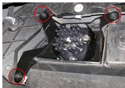
4. Install your assembled bracket and pod onto the vehicle by securing the three original bolts with a 7mm socket and ratchet.
